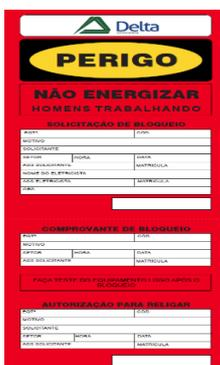
The form is titled 'PERIGO NÃO ENERGIZAR HOMENS TRABALHANDO' and includes sections for 'SOLICITAÇÃO DE BLOQUEIO', 'COMPROVANTE DE BLOQUEIO', and 'AUTORIZAÇÃO PARA REALIZAR'. It contains fields for equipment name, location, and dates, with checkboxes for 'OK' and 'NÃO OK' for various stages.
